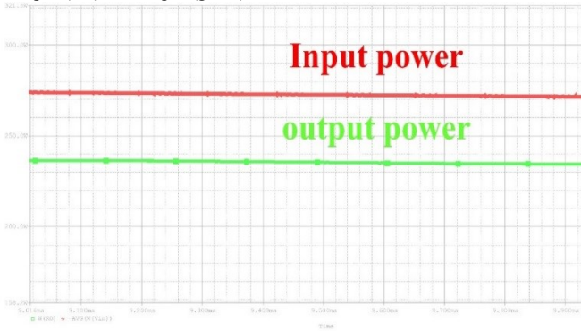
Fig 9. Exactly value of input (red) and output (green) of the DC-DC converter
