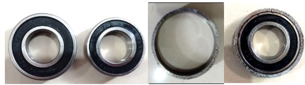
Fig. 6. a) Comparison of normal bearing sizes with replacement bearings, b) Replacement bearings with eccentric rings.
