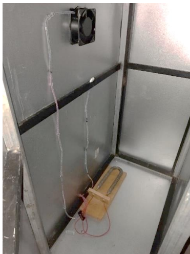
Fig. 8 Placement of Heater and Exhaust Fan
