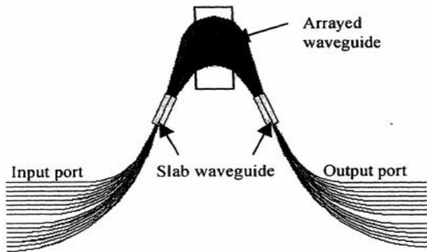
Fig. 3. AWG Basic Components
