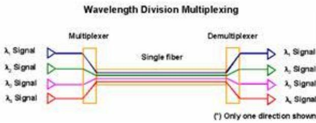
Fig. 2. The Concept of WDM
