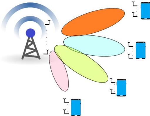
Fig. 1. Illustration of Multi-user MIMO Model
