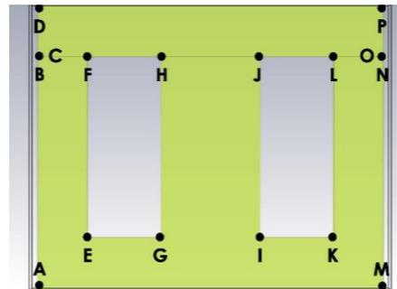
Fig. 3. Monitor locations on transformer
