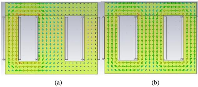
Fig. 7. Magnetic field density distribution of 0.03 cm laminated core at phase 0° (a); and 60° (b).
