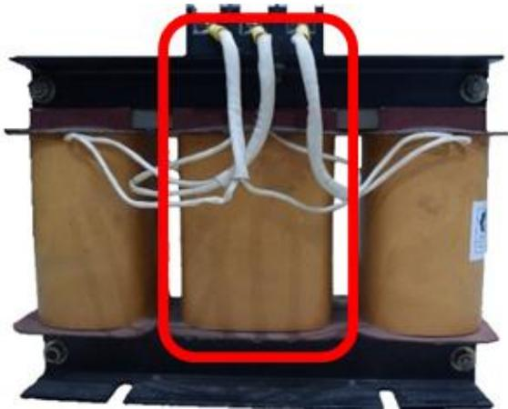
Fig. 1. Asymmetrical three phase transformer
