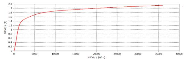
Fig. 4. Magnetization curve of ST-37 steel material
