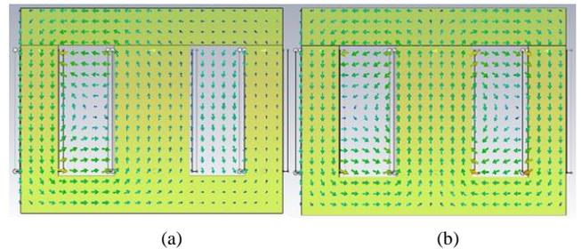
Fig. 8. Magnetic field density distribution of 0.03 cm laminated core at phase 300° (a); and 330° (b).
