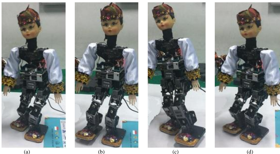
Fig. 5. Test of Walking Movement. (a) Preparation of right leg swing phase. (b) Swing phase with right leg. (c) Swing phase with left leg. (d) Standing phase.
