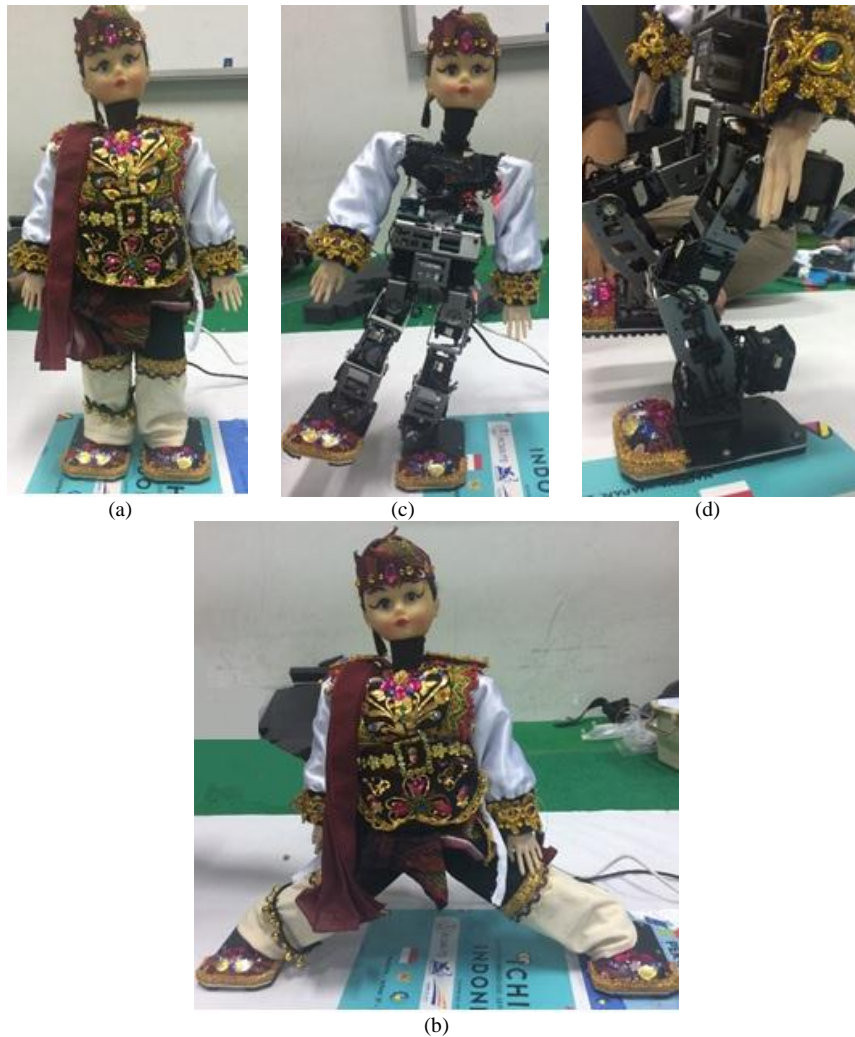
Fig. 6. Flexibility and foot lifting test. (a) Stand condition. (b) Stance phase to test how far leg widen. (c) Front view of foot lifting test. (d). Side view of foot lifting test
