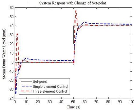
Fig. 15. Three-element control's response with change of set-point
