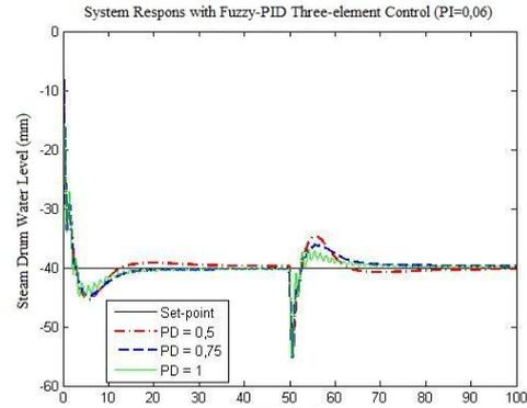
Fig. 14. System response with three-element control
