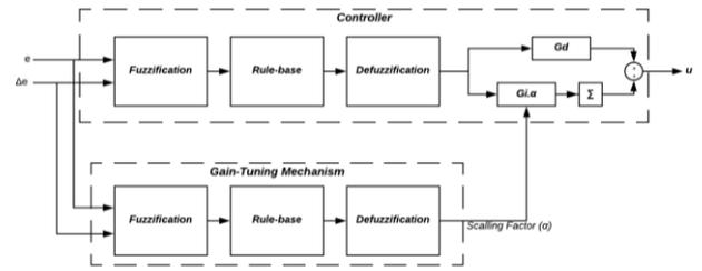
Fig. 3. Fuzzy-PID robust-self tuning controller
