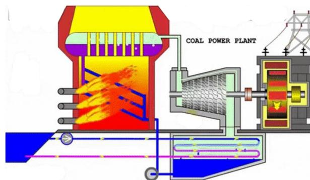
Fig. 1. Steam power plant work system [16]
