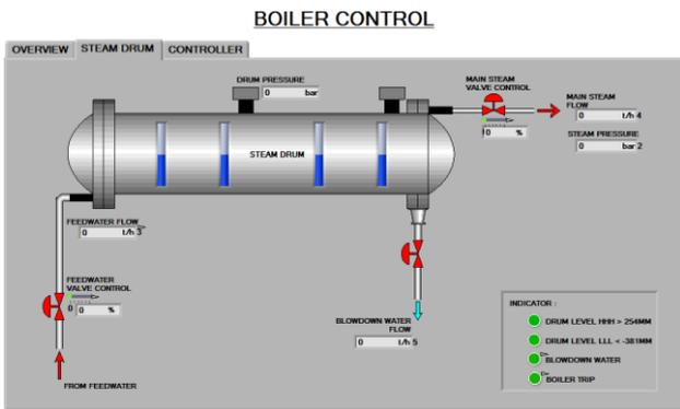
Fig. 8. HMI display in the Steam Drum's panel
