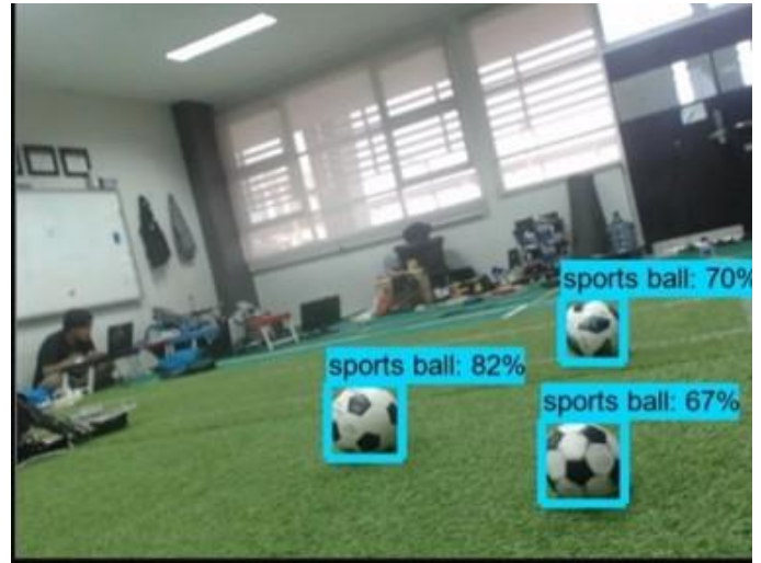
Fig. 5. An example of ball detection using deep learning.
