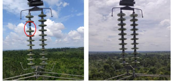
Fig. 2. Example of dataset, crack (left) and normal (right)
